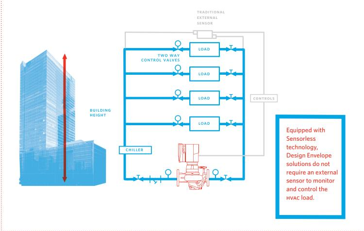
Using Sensorless technology, a Design Envelope pump's performance data (power draw and RPM) and operating curve are pre-programmed into the controller. During operation, the controller monitors the power draw and RPM of the pump and establishes the hydraulic performance and position of the pump's head-flow condition relative to the system requirements.
